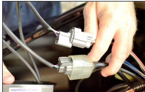
Secure Override Module "A" to OE wire harness with supplied zip ties. (2)
