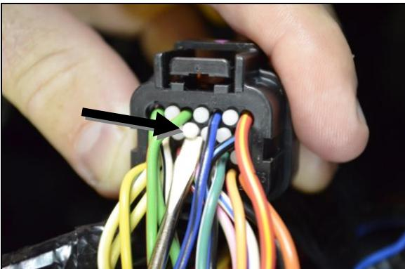
Insert wire with pin on Override Module "B" (smaller unit) into the #10 pin location of plug. Make sure it is installed completely.
